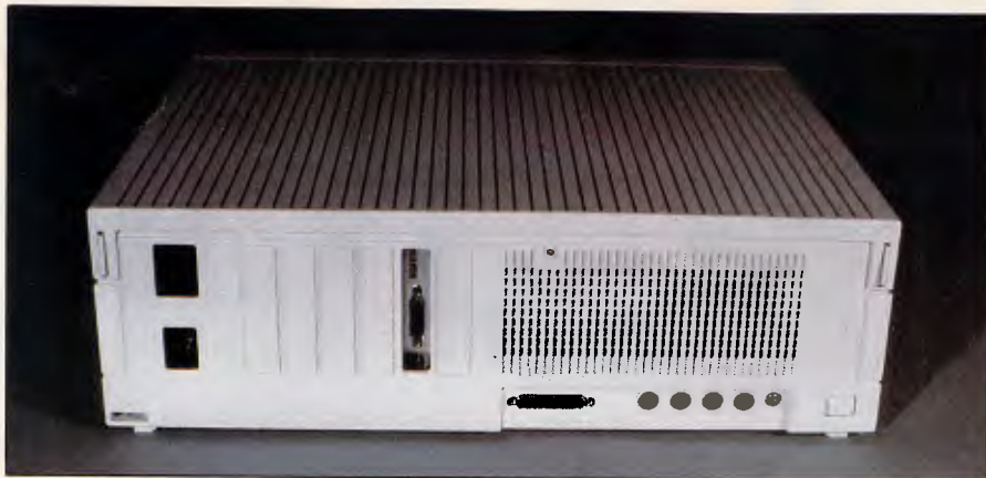
At the rear two 8-pin serial ports, handled by a Zilog 8530 controller, provide synchronous and asynchronous support for the Appletalk system
