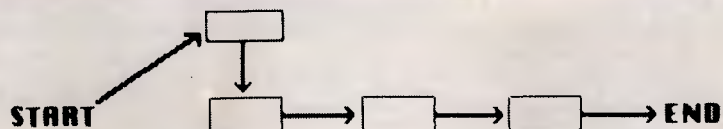
Fig 2 A singly-linked list with a new data item inserted between the start and the first data item. Only pointers have to be changed
