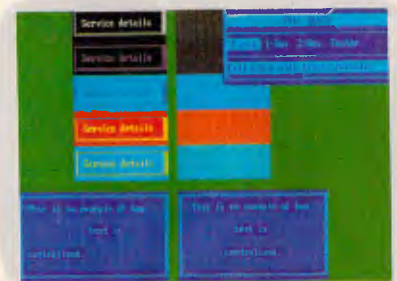
Each 'Service details' box is an overlay. The whole block was copied to the right and, as you can see, only the attributes moved
