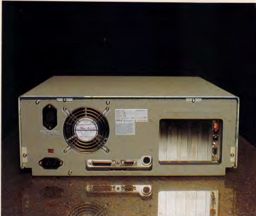
The Powermate has six slots: one 8-bit and five 16-bit
